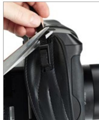
Using scissors, cut the remaining end of the strap and, to prevent unraveling, burn the tip of the nylon strap in order to seal the end.
