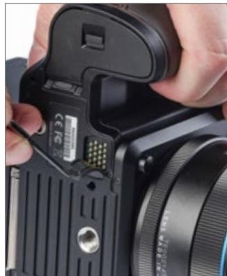
Remove the rubber cover from the electronic contacts by gently prying it from its recess.
