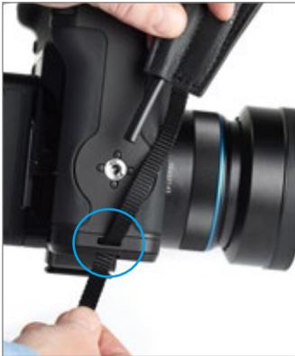
Ensure the side of the hand strap with the tube and the buckle is facing outward, away from the V-Grip. Thread the loose end of the strap through the bottom mounting point on the V-Grip. Thread it through the top opening first and out through the bottom opening, as shown.
