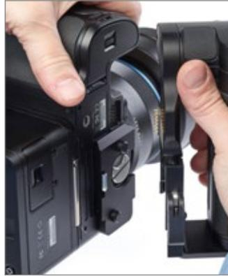
Make sure that the quick release on the V-Grip is open. The latch should point 90 degrees out from the grip. Place the V-Grip on the bracket on the XF camera body so it aligns with the XF hand grip and the contact pins integrate well into the connector recession.
