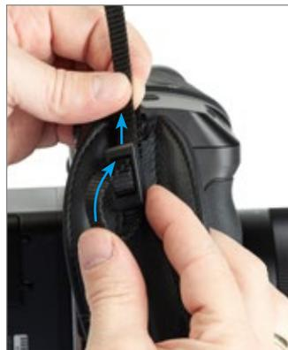
In order to secure the hand strap as much as possible, thread the strap back through the top end of the buckle and then pull to fasten it.
