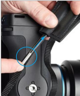
Push the supplied pin into the tube in order to make sure that the strap is attached firmly to the tube. This step is important to ensure that the strap can be guided from one end of the hand strap channel to the other.
