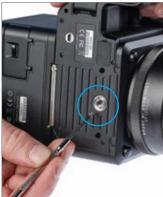
Use the supplied screwdriver and remove the small retaining screw from the tripod mounting socket of the XF camera body. Make sure to store the screw a safe place, as you will need it again if you want to secure the tripod thread adapter later on.
